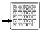
If you press an incorrect function key (+, –, ×,  $\div$ ), simply press the correct key and continue.
